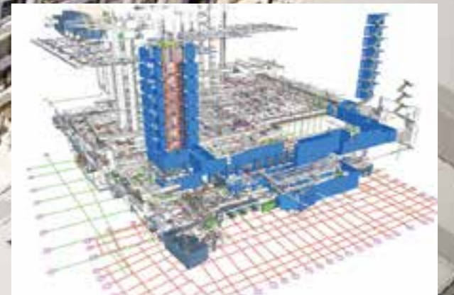
Clash detection within the federated model produced by One
